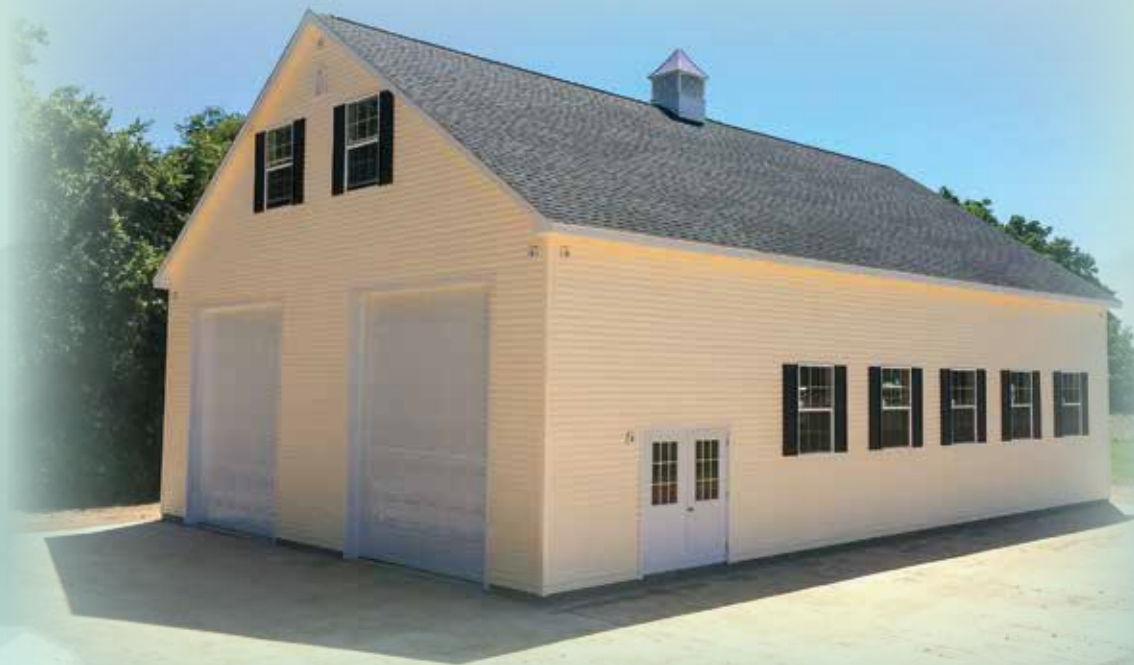
40x60 One-Story A-frame 20x60 attic trusses, cream vinyl siding, white trim, black raised panel shutters, black roof, two 14'x12' white garage doors, 40x60 windows, 8/12 roof pitch, 15' walls, 36" classic series cupola with concave copper roof
